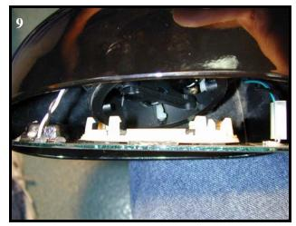
Tuck the wires toward the back of the mirror housing. Align the *Signal*<sup>®</sup> mirror over the center hub of the mirror housing and firmly press the mirror into the housing until it snaps into position.
